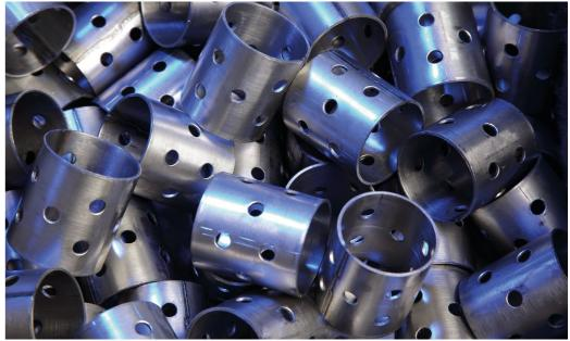
The manufacturing of rings, bushes and sleeves can be carried out efficiently and economically with the aid of punching-bending technology. Here a strip of metal is cut to length and bent around a core. The two ends stand in front of one another in the form of a slot or are joined by clinching.
